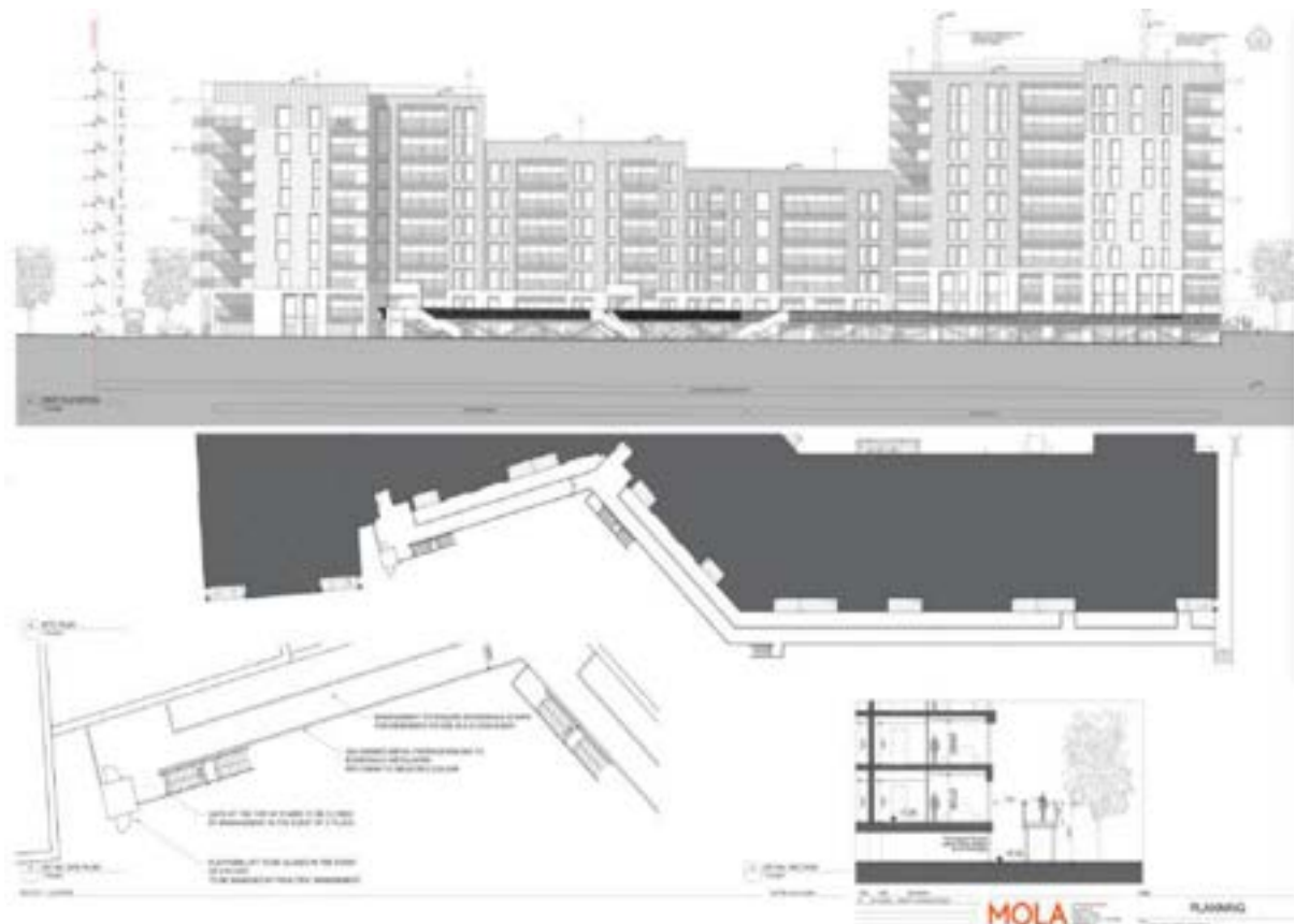
Figure 1: Section and Plan details illustrating primary flood mitigation comprising boardwalk & raised FFL
