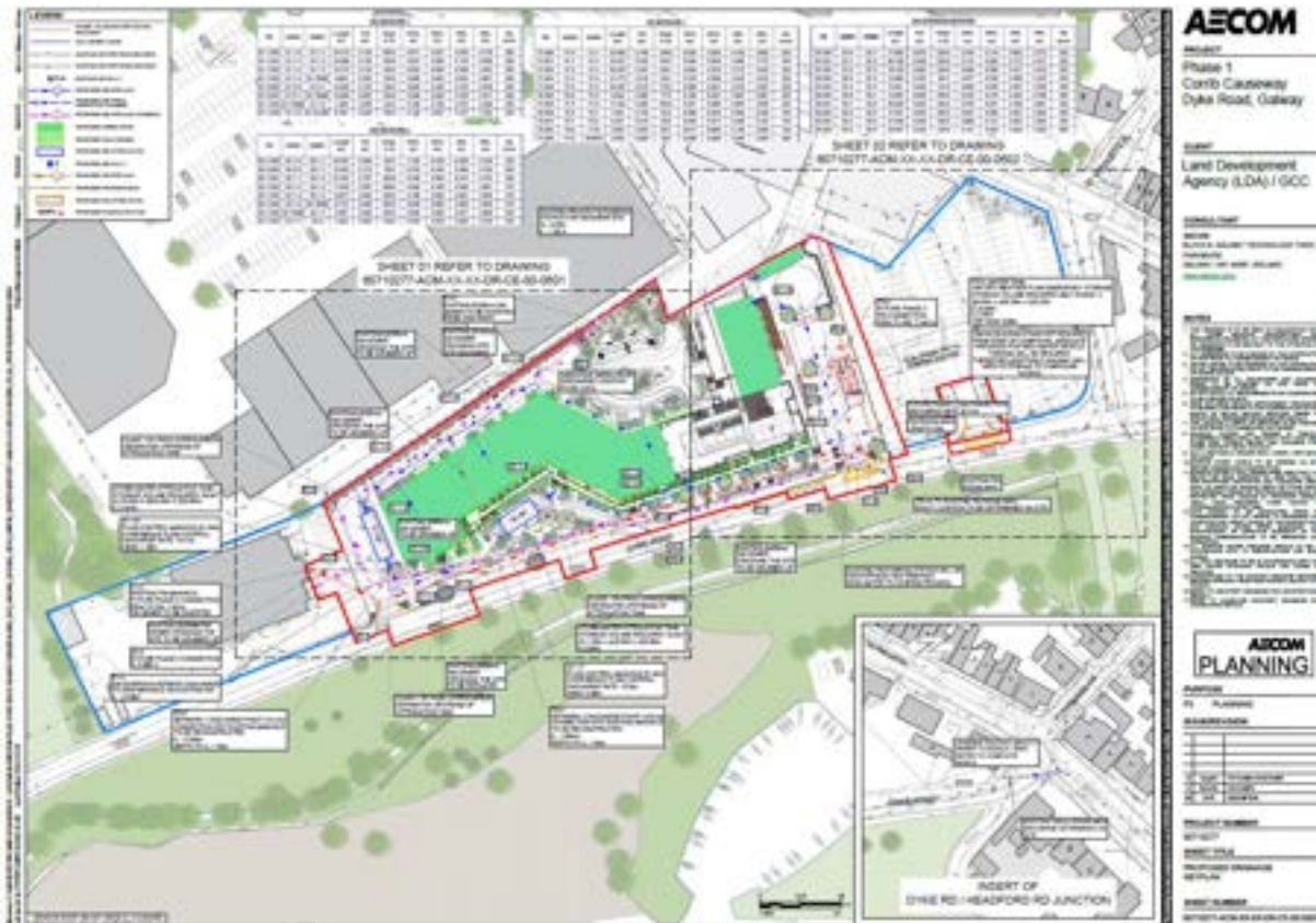
Figure 3-2. Proposed Drainage Layout (AECOM, 2025a. Proposed Drainage Keyplan)
