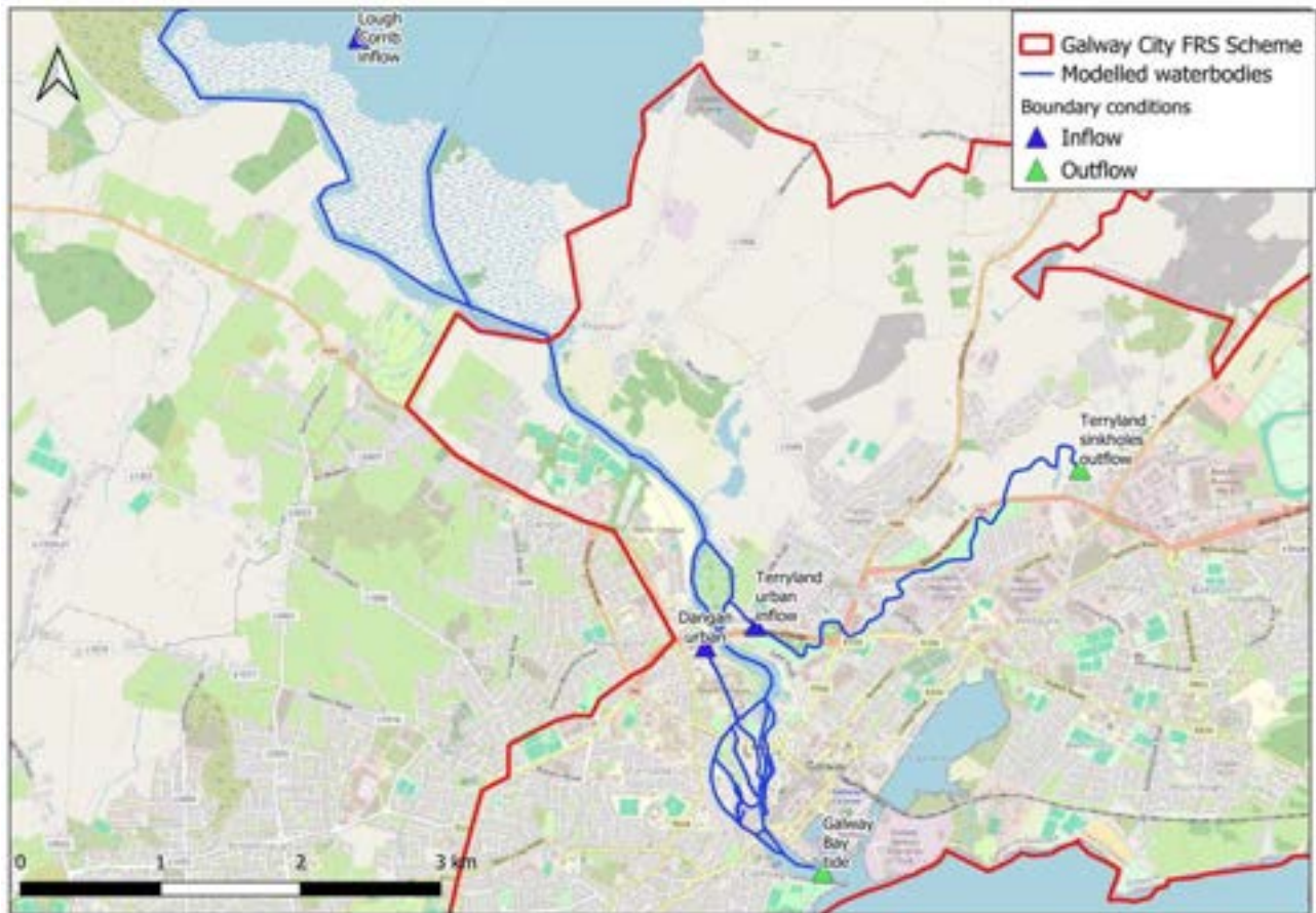
Figure 5 Fluvial/tidal model – model boundaries
